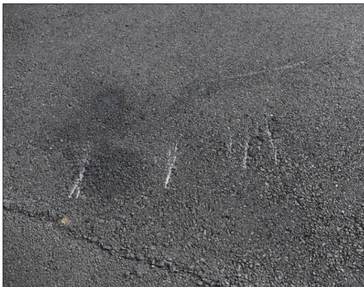
Photo No. 3: Propeller marks in paved surface where aircraft came to a stop
