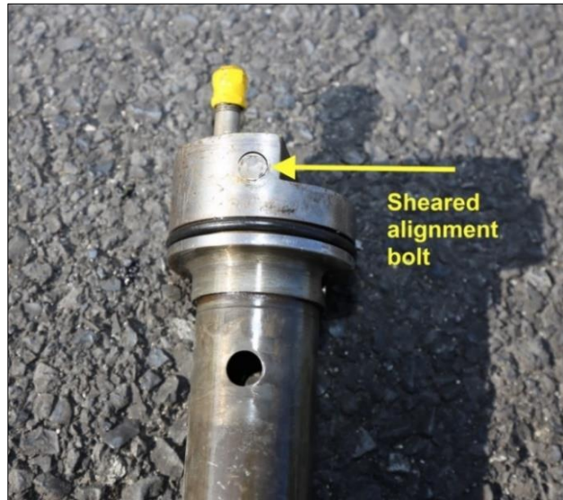
Photo No. 1: Sheared alignment bolt at top of oleo assembly
